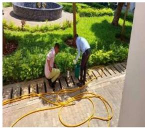
Plate No. 4.1-2: Water Sampling for Laboratory Analysis for a Water tap found at the Garden IMS Administration Building.
