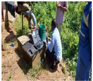
Plate No. 4.1-1: In-situ Water Quality Examination for Shakanii Drilled Well. Source: (Field Survey, June 2023)
